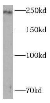
A431 cells were subjected to SDS PAGE followed by western blot with FNab09750(ZO1 antibody) at dilution of 1:1000
