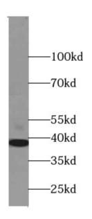
HepG2 cells were subjected to SDS PAGE followed by western blot with FNab08347(STOML2 antibody) at dilution of 1:1000
