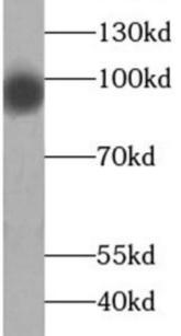
A549 cells were subjected to SDS PAGE followed by western blot with FNab07984(SLITRK6 antibody) at dilution of 1:500
