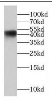
PC-3 cells were subjected to SDS PAGE followed by western blot with FNab06708(PPP1R7 antibody) at dilution of 1:1000
