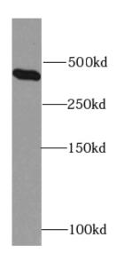
COLO 320 cells were subjected to SDS PAGE followed by western blot with FNab04063(HSPG2-Specific antibody) at dilution of 1:300
